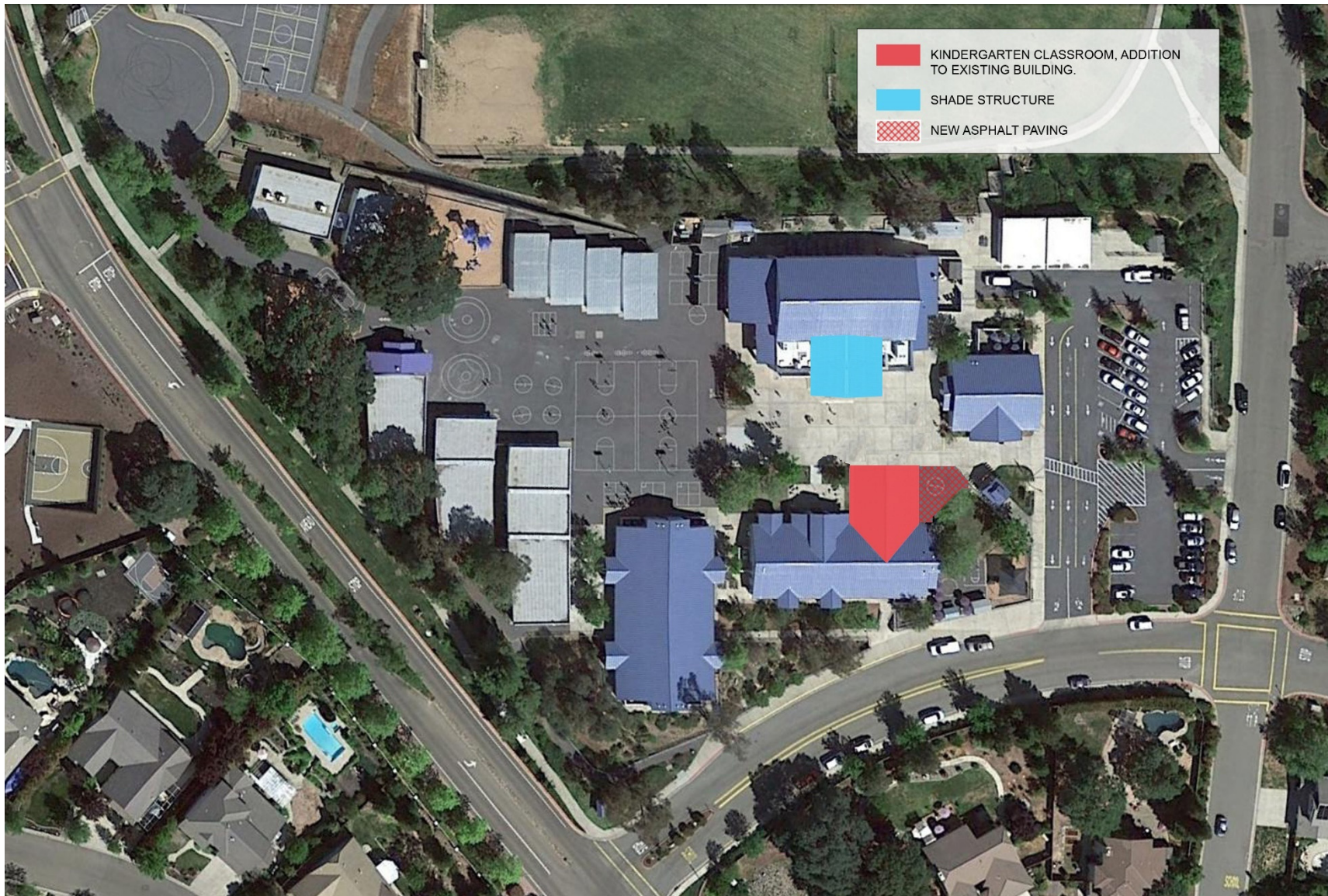
SCOPE OF WORK – PHASE 1 – KINDERGARTEN ADDITION / SHADE STRUCTURE LAKE FOREST ELEMENTARY SCHOOL
